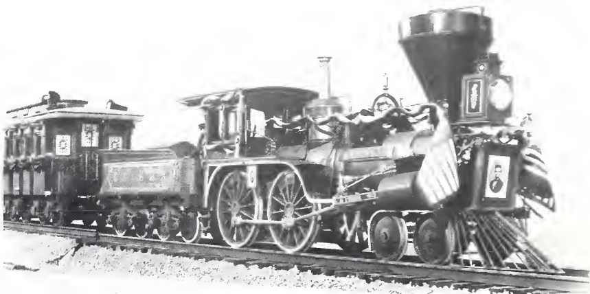
The model locomotive "Nashville" carries the same bunting and flags as the original. It was made from a three inch diameter plastic water pipe with many special urethane plastic castings. (W. Wesolowski)
