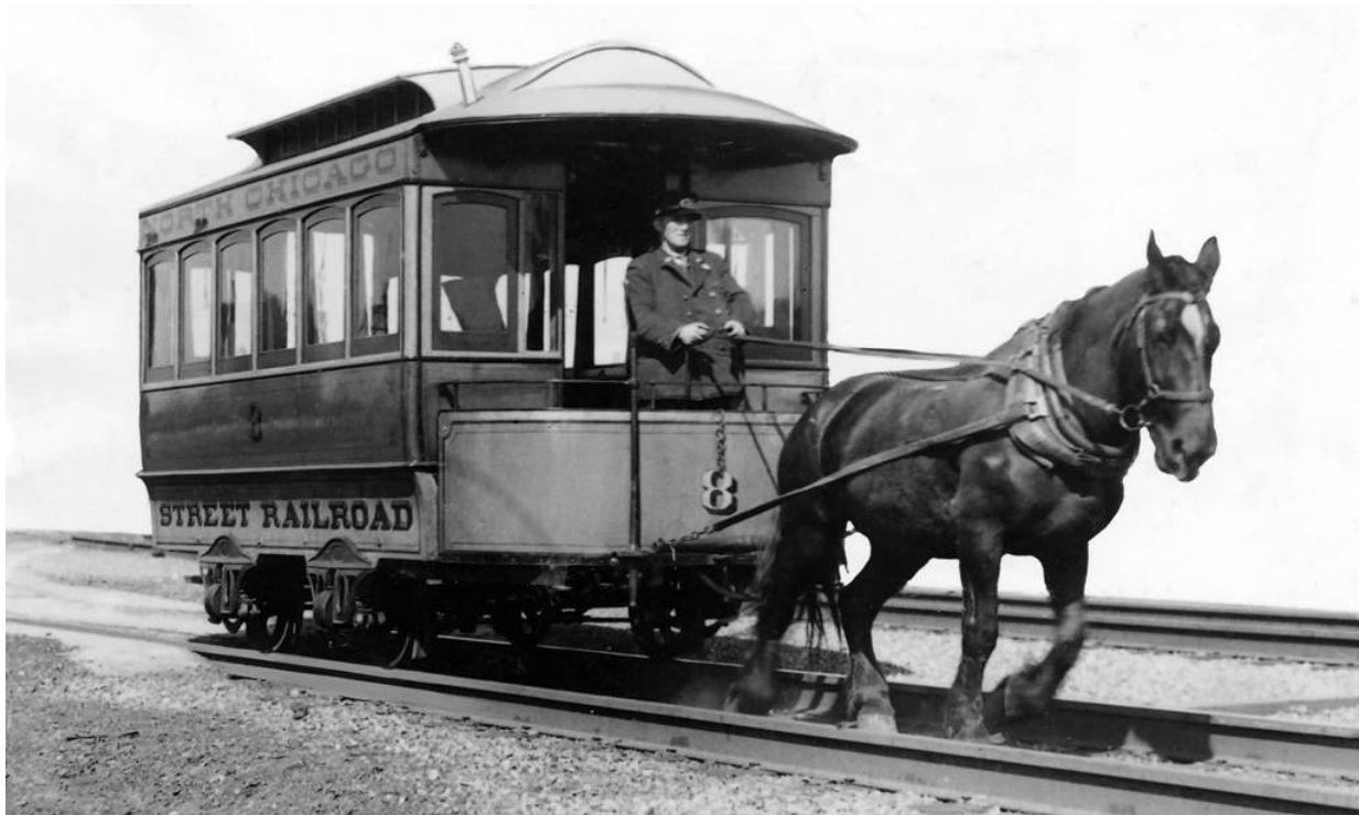
Chicago's first one-horse drawn streetcar ran along State Street from Randolph Street to 12th Street. The car was called a "Bobtail", having no rear platform.
