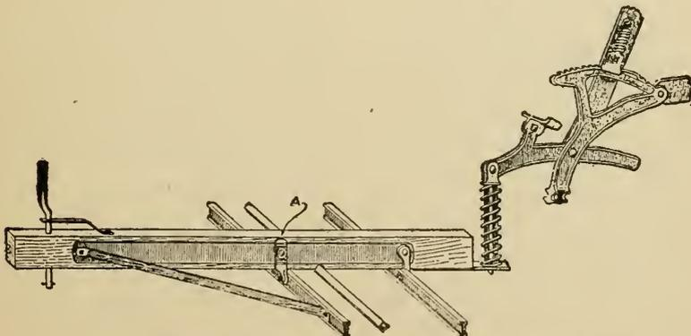
Fig. 1. Tongue Adjustment to Secure Accurate Checking
