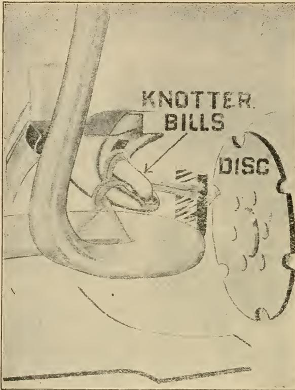
similar in position. This is particularly true in the knotter head or that portion of the binder head which ties the knot. In discussing these troubles then, let us bear in mind that every make of binder has in some form each part shown in the second illustration, and that the functions of these parts are the same though the position and shape may vary slightly.
