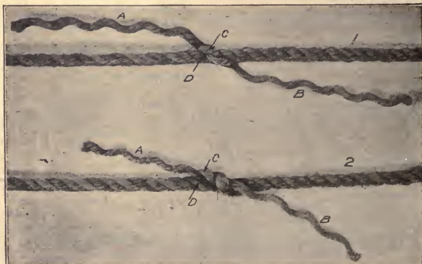
Fig. 6. Tying Ends in Repairing a Broken Strand and in the Long Splice.
