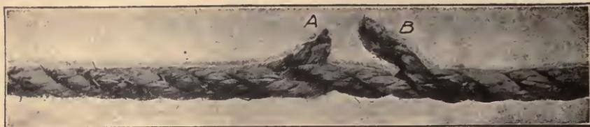
Fig. 1. A Broken Strand to Be Repaired.
