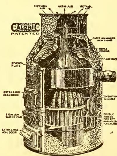
A furnace with no pipes. Think of it! Stands in the cellar directly under the register and pours heat up through all the house, warms the farthest corner and maintains a temperature there, but two or three degrees less than in the room where the register is. Very economical too. Positively guaranteed to save at least one third of your fuel —coal, coke or wood.
