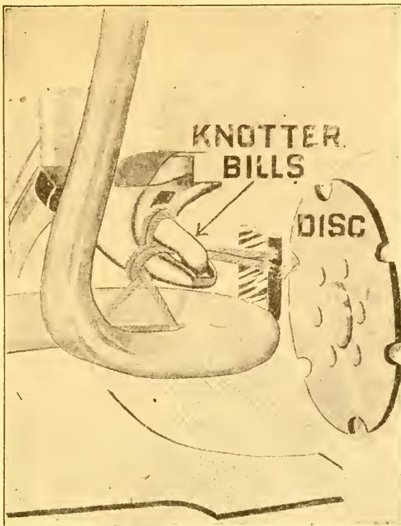
similar in position. This is particularly true in the knotter head or that portion of the binder head which ties the knot. In discussing these troubles then, let us bear in mind that every make of binder has in some form each part shown in the second illustration, and that the functions of these parts are the same though the position and shape may vary slightly.
