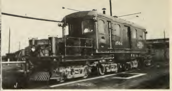
ITS pioneered in the development of the four-truck articulated locomotives of types C (above) and D (lower half of page).
